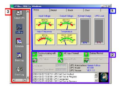
Section 1 is the UPS Dynamic Display Area where relevant information regarding the UPS is displayed. Selection of different display modes is possible, with information including input voltage, output voltage, line frequency, battery capacity, load, temperature, etc.
